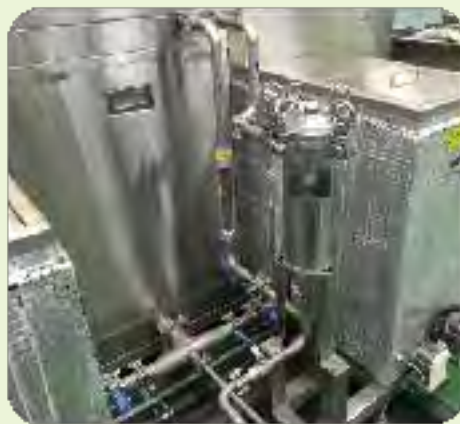
Installation of treatment facilities to increase the number of water cycles (Backflush-type rinsing tanks reduce water consumption and increase wafer cleanliness, supplied water can be recycled and reused)
