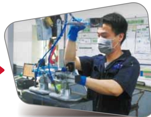
Addition of an effort-saving wafer suction device to reduce the workload during the transportation process and lower the risk of injuries
