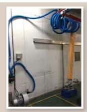
To ease the personnel off the loading/unloading of weight, pneumatic labor-saving racks are added to replace manual loading/unloading.
