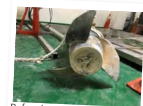
Before improvement - the mixer blades were seriously worn.
