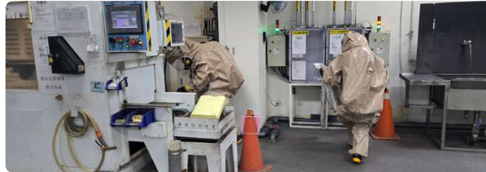
4. The Emergency Rescue Team enters the hot zone: (1) Operate the equipment to stop the acid discharge and contain the leak (2) Place absorbent pads and booms around the leak. (3) Once no residual liquid remains at the leakage site, place the used absorbent pads and booms into hazardous waste disposal bags.
