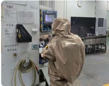
4. The Emergency Rescue Team enters the hot zone: (1) Operate the equipment to stop the acid discharge and contain the leak (2) Place absorbent pads and booms around the leak. (3) Once no residual liquid remains at the leakage site, place the used absorbent pads and booms into hazardous waste disposal bags.
