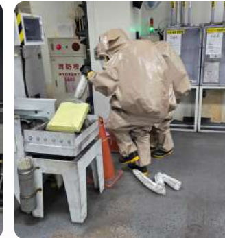
4. The Emergency Rescue Team enters the hot zone: (1) Operate the equipment to stop the acid discharge and contain the leak (2) Place absorbent pads and booms around the leak. (3) Once no residual liquid remains at the leakage site, place the used absorbent pads and booms into hazardous waste disposal bags.
